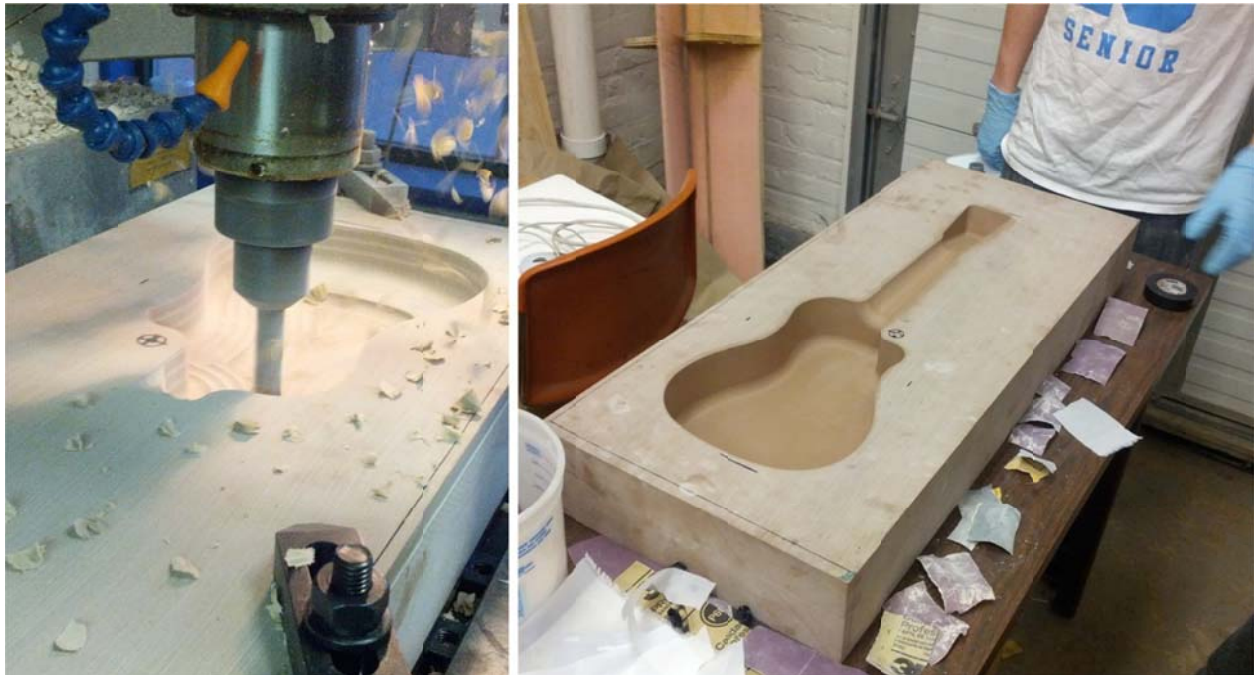
Figure 21 - CNC Machined Body Mold
