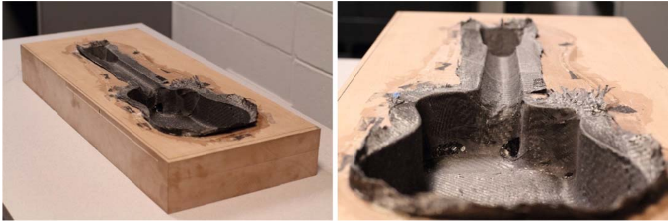
Figure 22 - CF Body Piece in Mold
