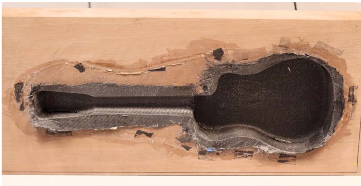
Figure 18 - CF Body Piece in Mold
