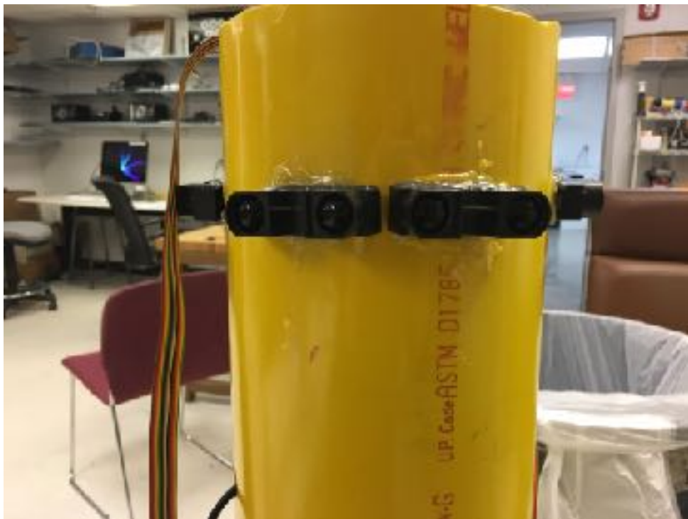
figure 4. hot glue, though ugly, gave us the best adhesion since the sensors were somewhat too delicate to clamp securely
