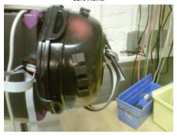
The left hand allowed the user to play chords with ease. Similarly to the right hand holes were poked in order to easily insert the four nodes of each button. Once the buttons were inserted wires were soldered to the upper right and lower left nodes of each button. Five momentary switch buttons were then inserted allowing the user to choose between playing the lower fifth, root, third, 5<sup>th</sup>, or whole chord. Again this bowl was cut into using a dremel in order to put on the straps.
