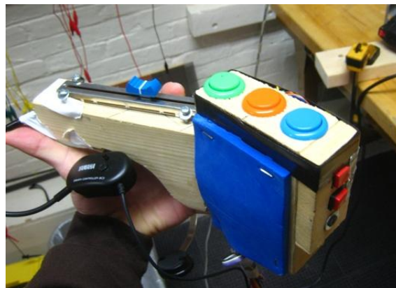
Figure 1- Right side of the trumpet controller. The accelerometer is located beneath the blue foam sheet.
