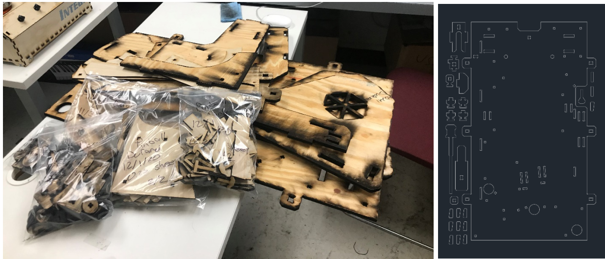
Figure 1 (left): Plywood pieces after laser cutting Figure 2 (right): Screenshot of one DXF for laser-cutting (four total)
