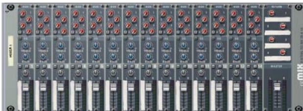
This is a mixer with fourteen stereo channels, four stereo effect sends and a basic two-band EQ section. By connecting the different devices to different mixer channels (and the stereo output of the mixer to the hardware interface) you can listen to all your devices at the same time, adjust levels and pan, add effects and so on - just like on a physical mixer.
