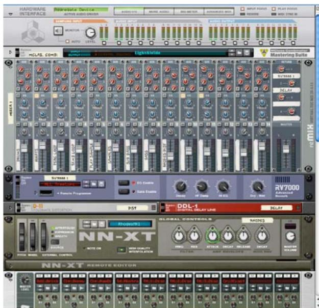
This is the virtual rack, the heart of Reason. At the top of the rack you will always find the Hardware Interface, which allows Reason to communicate with the audio hardware. Below this, you can add as many different devices you want (or as many as your computer can handle). Read more about the different devices below.
