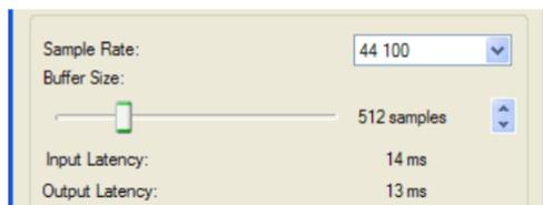
The Input Latency is the delay between when the audio is "sent" from a connected microphone or instrument and when it's received and detected by Reason. Output Latency is the delay between when audio is "sent" from Reason and when you actually hear it. The latencies in an audio system depends on the audio hardware, its drivers and their settings.
