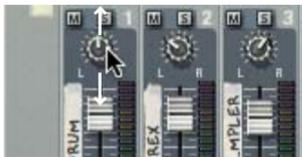
You may also want to add some effects to the music. In this song, there are two effect devices connected: a delay and a chorus/flanger. These are connected as send effects from the mixer, allowing you to specify how much of each mixer channel signal should be sent to each effect.
