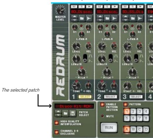
5. Try out the drum sounds by clicking the audition buttons at the top of each drum sound channel.
