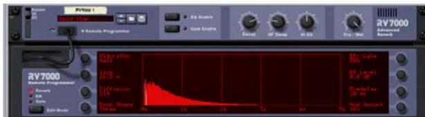
The RV7000 is a high quality reverb processor with nine different reverb and echo algorithms, ranging from rooms and halls to special effects. The RV7000 also contains an equalizer and a gate section, making it possible to get virtually any kind of reverb character, including gated reverb.
