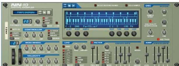
The NN-19 allows you to sample and to load samples (Wave, AIFF, SoundFonts or REX files) and create multi-sample patches by mapping samples across the keyboard. Once you have loaded one or several samples, you can modify the sound using synth-type parameters such as a filter, envelopes and an LFO.
