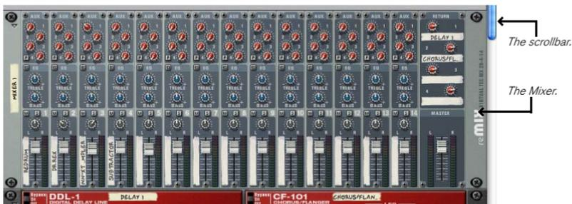
If you look at the mixer, you will see that each mixer channel has a "tape strip" next to the volume fader. If a device is connected to a mixer channel, the tape strip is labeled with the device name. In this song, there are only four instrument devices, so only the four first mixer channels are labeled.
