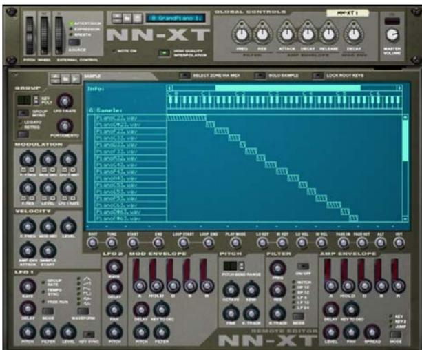
The NN-XT - just like the above mentioned NN-19 - lets you sample and load samples (Wave, AIFF, SoundFonts or REX files) and map these across the keyboard to create multi-sample patches. The sound can then be modified using synth-type parameters; two LFOs, two envelopes and a filter.
