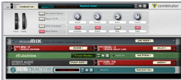
The Combinator allows you to create new "custom" devices by combining existing devices. Any combination of Reason devices can be added to the Combinator and then saved as a "Combi" patch. Example usage includes creating layered instruments, instrument/effect combinations and effect chains. Devices in a Combi can be mapped to velocity/key zones and the Combinator also features virtual knobs and buttons that can be assigned to any device parameter or function.
