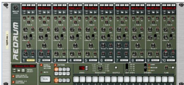
The Redrum is a sample-based drum machine with ten drum sound channels. You can sample and load samples (Wave, AIFF, SoundFont files and REX slices) individually for each channel, or open patches, which are complete drum kits (a number of which are included in the Reason Factory Sound Bank). Each sound channel has settings for pitch, level, velocity response, etc.
