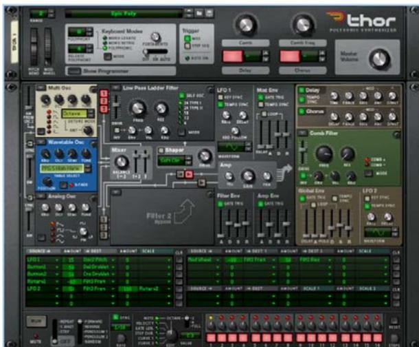
Thor is an advanced semi-modular polyphonic synthesizer based on various selected vintage synth designs. It features several different oscillator and filter-types which can be loaded into open "slots", allowing for an incredible tonal variety. It also has an extensive modulation section and an advanced "analog-style" Step Sequencer.
