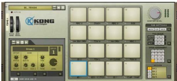
The Kong Drum Designer is an advanced drum sound module with 16 drum sound channels. You can sample and/or load samples (Wave, AIFF, SoundFont files and REX files) individually for each channel, or open patches, which are complete kits (a number of which are included in the Reason Factory Sound Bank).
