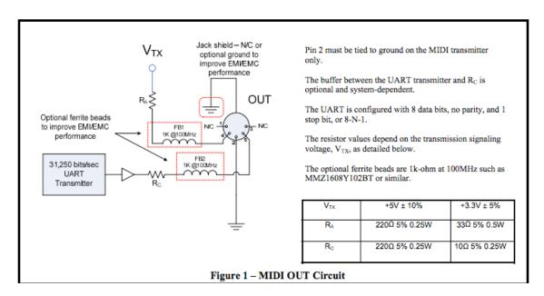
The MIDI signal is on Pin 5 of the connector, and the voltage to drive the circuit (see Figure 1) is on Pin 4. Pin 2 is connected to the cable shield, and Pins 1 and 3 are not normally connected.
