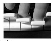
**An**H is **Polyphonic Key Pressure**, sometimes known as polyphonic (or just "poly") aftertouch. It is similar to Channel Pressure, except that each note has an *independent* sensor, and can be addressed individually. It allows, for example, vibrato or a timbral change to be applied to one note in a chord but not the others. A Polyphonic Key Pressure command has two data bytes: the note number, and the amount of pressure.
