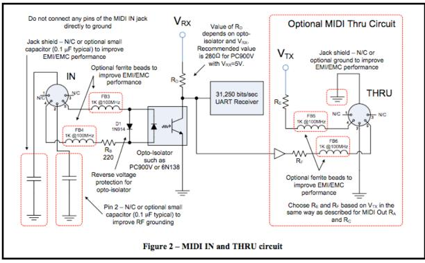
The optoisolator is commonly connected to a chip known as a "UART," for "Universal Asynchronous Receiver/Transmitter." The UART translates the MIDI pulses into a form that the receiving device can understand. In a MIDI transmitter it works the other way around: the UART takes data from the synthesizer and makes MIDI out of it.
